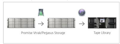
**Step 1 – Cloning to Disk:** One of the safest strategies for data availability and safekeeping is combining failover and backup and creating a diskto-disk-to-tape setup. In this scenario, P5 Synchronize mirrors data from the primary online storage to a secondary online storage for an identical copy of data that is immediately available.
