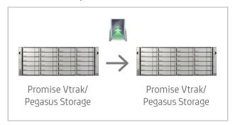
Shared production storage is time critical. It needs to be kept available all the time. Archiware's P5 Synchronize clones data to the secondary storage, creating a failover solution on the secondary storage. In case of emergency, switching over takes only minutes before all data is again available to continue production. Additionally, file versions and snapshots can be kept.
