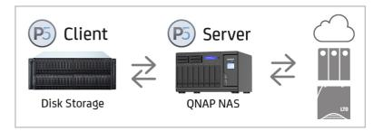
Data from QNAP devices is stored in a platform neutral format including user authorizations - identical to all other supported platforms. Archiware P5 runs on QNAP NAS devices with the QTS operating system 4.3+ and an Intel x86 64-Bit processor.
