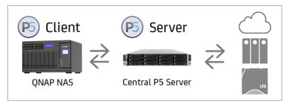
Archiware P5 can be combined with a QNAP NAS using two different setups. In the first setup, P5 acts as a central server, which synchronizes, backs up and clones data from the QNAP NAS onto the desired target (disk, tape or cloud). The QNAP NAS is connected to the central P5 server as direct attached storage or as a P5 client.
